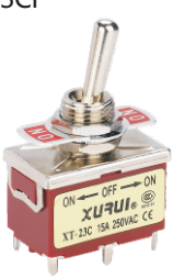
·双极双向自动复位型 DPDT Auto Reset (ON)-OFF-(ON) XT-23CF
